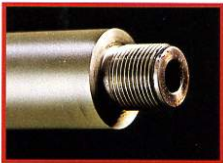
A removable cap protects the rifle's threaded muzzle (shown) that can accept a variety of suppressors or muzzle brakes.
